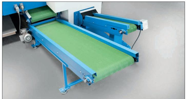
Double conveyor to unloading point
